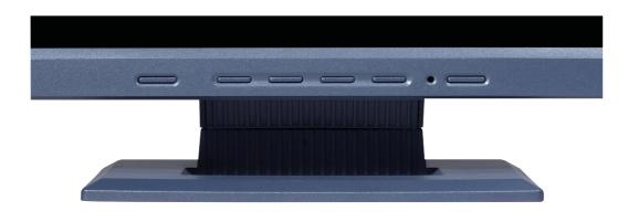
There are 6 keys for user's control including "*iKey*", "Exit", "Enter", "<" and ">" key and a power swith. The following descriptions are the introduction of these keys & switch.
